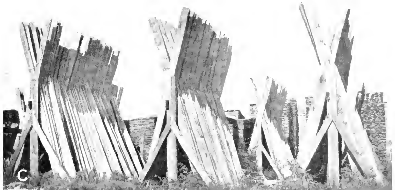
Some methods of piling other than flat: A, Lumber end piled on a solid wooden platform. An open foundation for each pile, raised a foot or more above the ground, would afford better air movement around the bottom of the pile; B, a rack for the end piling of lumber; C, yard lumber end racked in the form of an X
